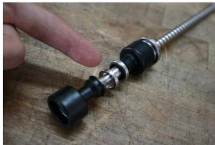
7. Slide (1) rubber boot over the other end of connecting rod with metal collar facing out, and secure in place using retaining ring.
