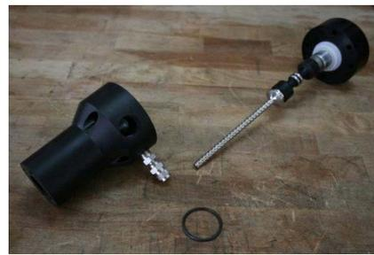
6. See (2) black rubber boots on connecting rod. Slide back metal collar on rubber boot to reveal (2) metal pins connecting pump rod/shaft assembly.
