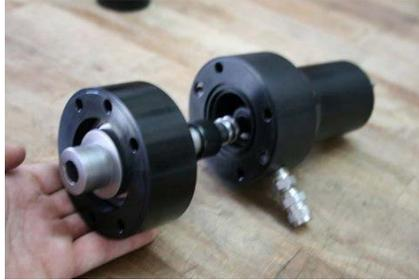
12. Press lower bearing plate firmly to pump body, making sure white plastic seal is seated into pump body.
