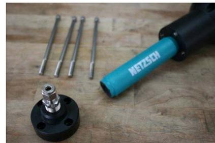
17. Place the plastic stator flange on the end of the pump stator and ensure the stator fits securely into the counter-bore on the stator flange, then Insert (4) 1/4-20 X 5.5" screws through stator flange and thread screws into the pump body.
