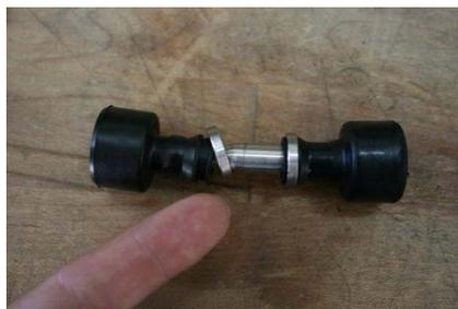
9. Remove (2) rubber boots from connecting rod.
