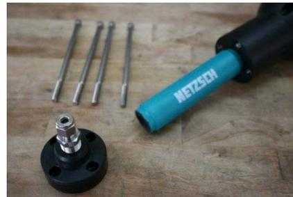
2. Carefully pull and unwind (counter clock wise) pump stator from rotor.
