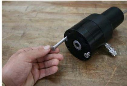
4. Carefully remove upper bearing plate.
