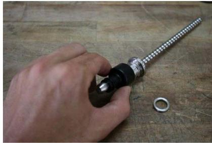
5. Use (1) metal retaining ring to secure rubber boot to connecting rod.
