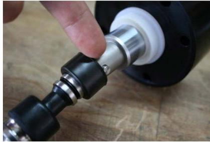
9. Make sure both rubber boots are securely in place covering metal pins in through holes.
