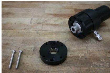
5. Carefully pull lower bearing plate apart from plastic pump body. Dislodge white plastic seal, and rubber o ring from plastic pump body, and pull entire input shaft and pump rod assembly through the plastic pump body. (Keep white plastic seal secured to input shaft.)
