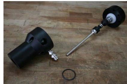
10. Install rubber o'ring into groove on plastic pump body.
