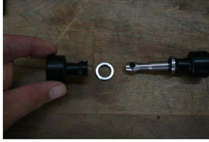
10. Remove white plastic seal from input shaft, and carefully remove input shaft from the lower bearing plate.
