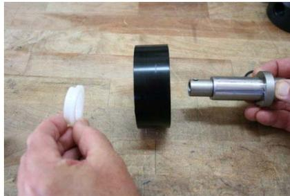
3. Insert connecting rod into pump rod, and secure with (1) metal pin through both holes in the input shaft.
