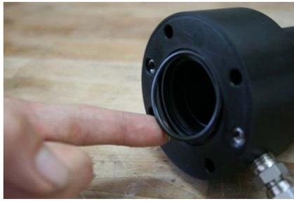
11. Very carefully insert pump shaft assembly through the pump body.
