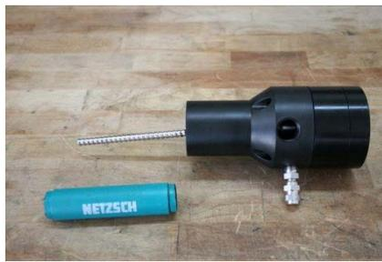
14. Secure top bearing plate, middle bearing plate, and pump body together using (2) 1/4-20 X 2.5" flat head screws.
