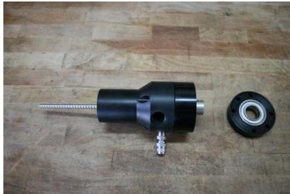
13. Carefully slide upper bearing plate over end of input shaft, securing upper bearing plate to the lower bearing plate.
