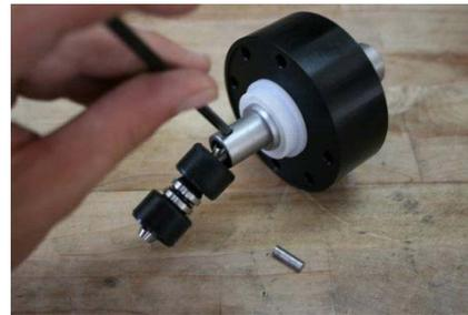
8. Carefully remove (2) metal retaining rings securing rubber boots to connecting rod
