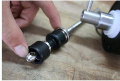
8. Insert end of connecting rod into input shaft, secure with (1) metal pin through both holes in the input shaft.
