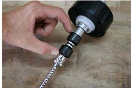
7. Remove (2) metal pins and detach connecting rod from pump rod and input shaft.
