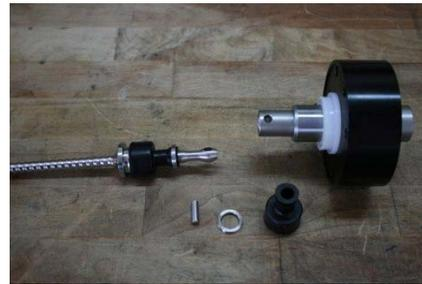
6. Slide (1) metal retaining ring over the other end of connecting rod.
