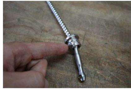
4. Slide (1) rubber boot onto connecting rod. Slide and secure rubber boot collar in place over metal pin.
